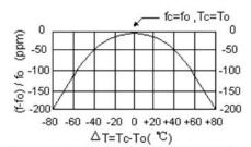
The curve shown above accounts for resonator contribution only and does not include LC component temperature characteristics.
