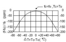
The curve shown above accounts for resonator contribution only and does not include LC component temperature characteristics.
