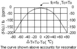
contribution only and does not include LC component temperature characteristics.
