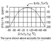
contribution only and does not include LC component temperature characteristics.
