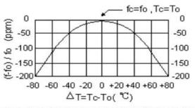
The curve shown above accounts for resonator contribution only and does not include oscillator temperature characteristics.
