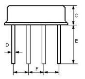
PinConfiguration1Input / Output4Output / Input2/3Case Ground
