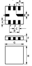
PinConnection2Input5Output1, 3, 6, 7to be Grounded4, 8Case Ground
