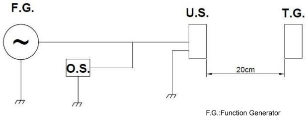
F.G.:Function Generator U.S :Ultrasonic Sensor
